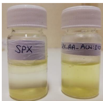
Figure 3-30 The comparison of solubility behaviour of Sparfloxacin (left) and SPX:AA (right)
